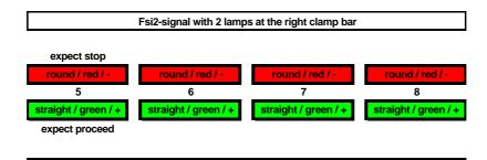
After switching-on the layout the light signal-decoder will switch at first both signals to the aspect "expect stop". On both signals the green LED will flash.
